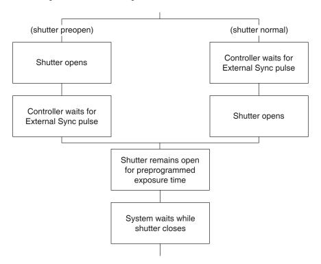
Figure 12. Chart showing Two External Sync Timing Options
